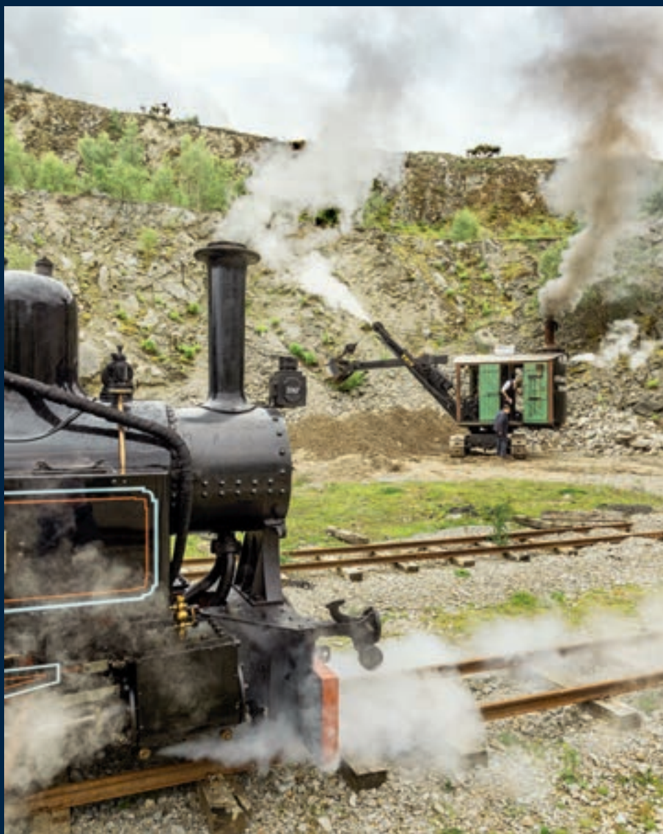
Quarry atmosphere: ex-Penrhyn 0-4-0T Marchlyn sneaks into shot, while US-built Erie 'Type A' steam shovel No. 3295 works in the background. Such 'steam navvies' were widely used before the advent of diesel-worked shovels. Gordon Edgar
