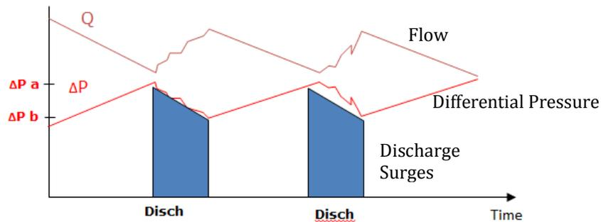
Having a single setpoint will maintain a consistent  $\Delta P$  in the baghouse, a consistent airflow through the mill and a consistent amount of material discharged, avoiding periodic overloading.
