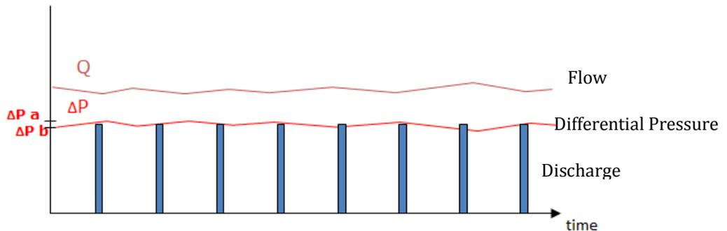
It's important to note that this recommendation does not result in excess pulsing. The system simply pulses when higher than 4.5" w.g. and stops if  $\Delta P$  is below 4.5" w.g. Sometimes it takes one pulse, sometimes two or three pulses. It essentially becomes a continuous pulsing program, but with variable time between pulses to stay at the programmed setpoint.
