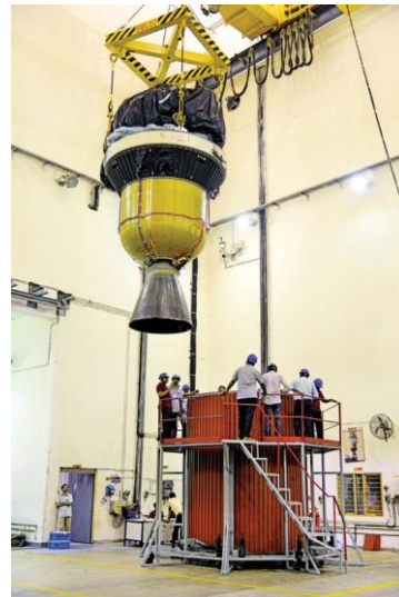
PSLV-C55 Third and Fourth stages at Stage preparation Facility
