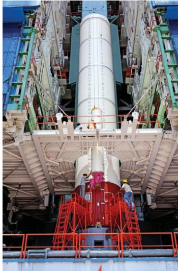
PSLV-C55 integration under progress at Mobile Service Tower
