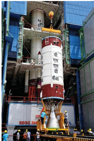
Hoisting of PSLV-C55 Liquid second stage
