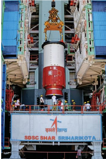
Hoisting of the nozzle end segment of PSLV-C55 first stage over the launch pedestal
