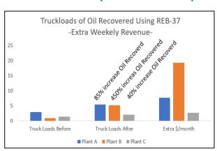
Oily water sent to SWD plants contained significant levels of hydrocarbons. Using NX Chemical BioBreak® REB-37 at <10 ppm enabled the recovery of significantly more oil, resulting in larger plant revenues and lower injection well impacts (plugging). The plot below shows the increase in oil recovered (40% to 450%) using BioBreak® REB-37 and the corresponding revenue increase per week (\$3K to \$8K) per plant.
