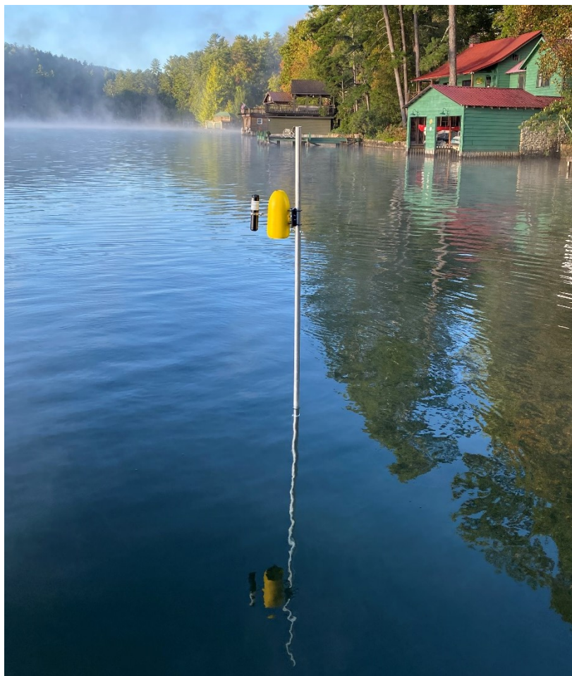
Figure 2-5. SonicXB gauge mounted to tripod in Lake Rabun
