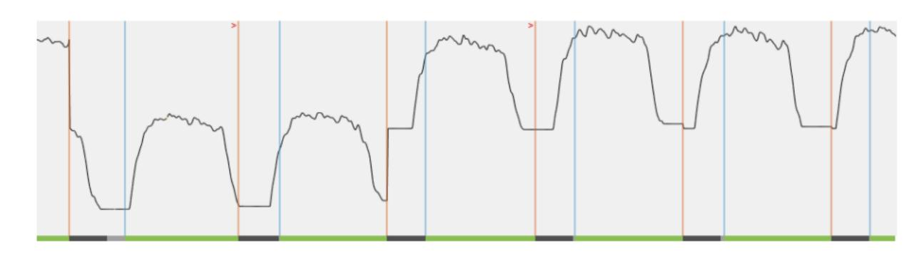
**Poor:** Noise and/or vascular signal more than 1/3rd of waveform amplitude
