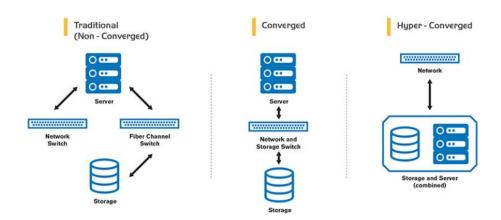
Hyper-Convergence in Network Hardware combines storage and processing power into a single appliance for simplified management, faster deployment, and could even lower acquisition costs (Helixstorm.com)
