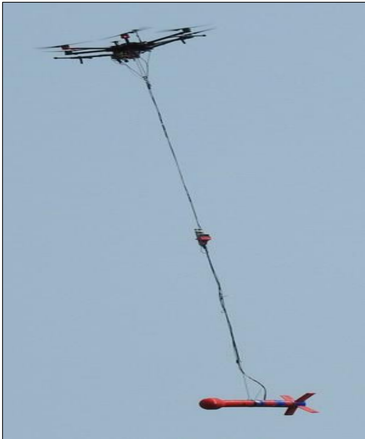
Figure 21: Devbriio UAV Multirotor drone with the CS-VL magnetometer used at Magusi West. Photo from the Abitibi Geophysics Logistic and Interpretation Report (Chemam, 2023).
