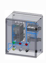
Integrated high resistance grounding systems are available in a panel configuration. These units contain controls, indication lights, touch screen panels, ground fault relays, current transformers, sensing resistors, resistors, and more.
