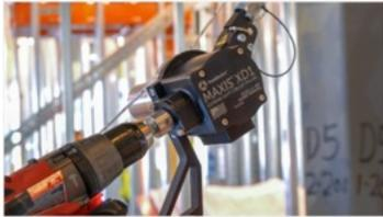
Safer, faster, and more efficient way to pull low voltage, branch home runs, lighting cables, and small circuit sized wires.
