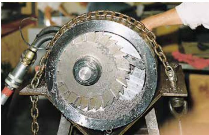
A Tri Tool custom manufactured portable saw with a rotary, eccentric feed that was designed to sever steel pipes that were encased in concrete, from the I.D.
