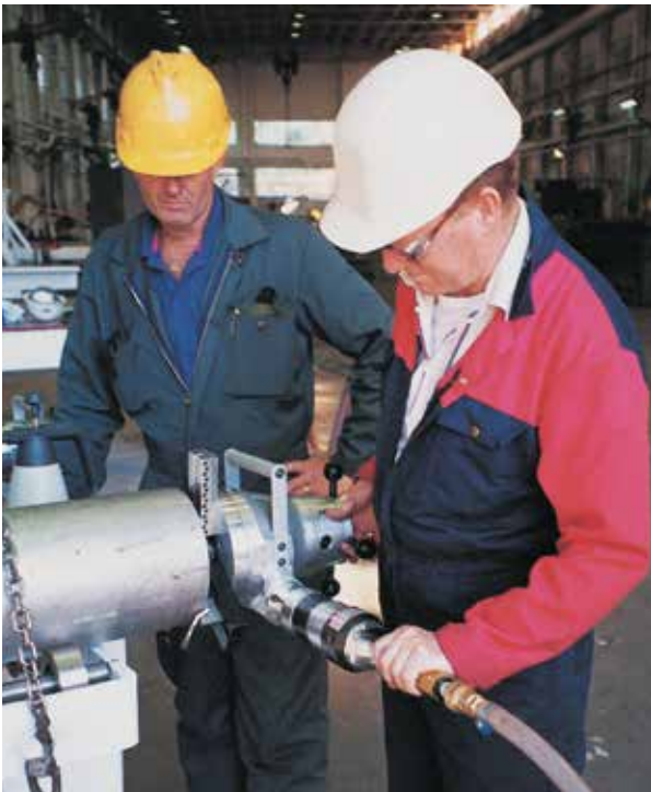
The dependable Model 214B BEVELMASTER being used in a fab shop to generate a precision form tool weld-prep end on stainless steel pipe.
