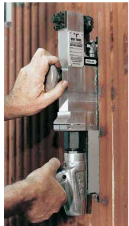
The narrow profile and well-designed controls make the Model 201BA BEVELMASTER the ideal solution for waterwall weld preps.
