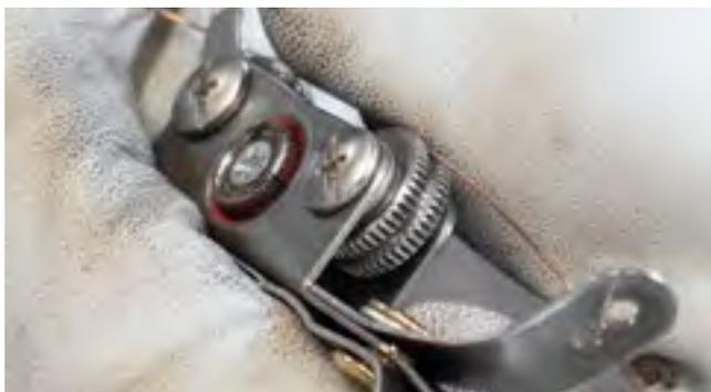
**CENTER GROOVE ON KNURLED THUMB WHEEL PREVENTS WIRE SHIFT.**
