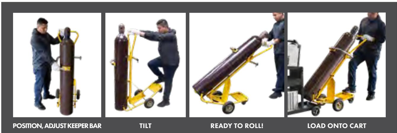
POSITION, ADJUST KEEPER BAR
