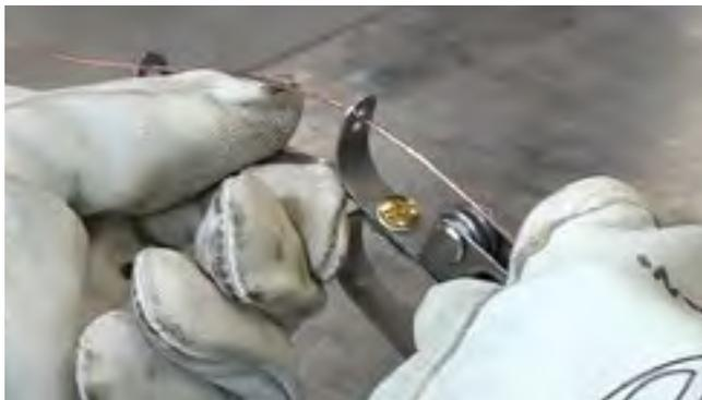
**BEND THE FEEDER ARM AS NEEDED TO CREATE WIRE TENSION AND STABILITY.**
