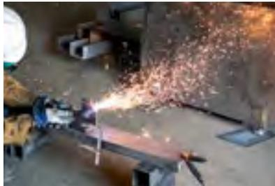
Setup a protective panel wherever needed to protect workers, equipment, and materials from heat, sparks, and slag.
