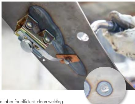
This handy, compact tool saves time and labor for efficient, clean welding of holes, joints, and seams in steel panels. Easy to use, even in tight, hard to reach spots.
