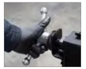
Two large handles for quick and easy adjustment of rotary axis
