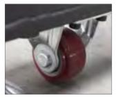
Two casters for quick repositioning of manipulator.
