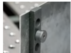
Magnet keeps sheet metal in vertical position
