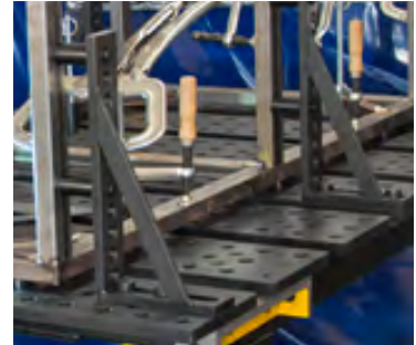
Insert V-Blocks to support round stock.
