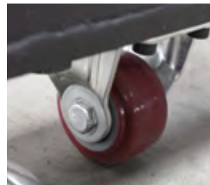
Two casters for quick repositioning of manipulator.
