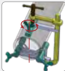
Turn three adjustment screws to preset.
