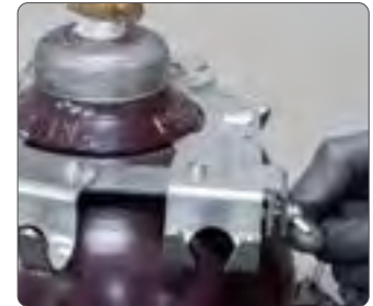
Thumb screw ensures a snug fit of the hooks on the cylinder.
