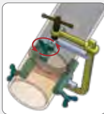
Tighten the main clamp arm.
