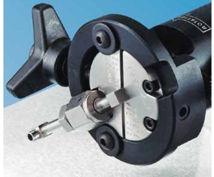
Special saddles for the Model 301SP include dedicated cutouts that correspond with recesses in the tool face to provide the perfect clearances required for squaring gland nut assemblies.
