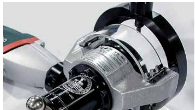
The 304's open design and integral, clear chip guard provide increased operator safety.
