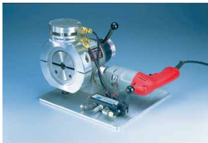
Tri Tool can modify stock tools for specific application requirements. This Model 302 has been configured with pneumatic saddle clamping actuation and a quick-detach air fitting for increased cycle times in a high volume tube production role.
