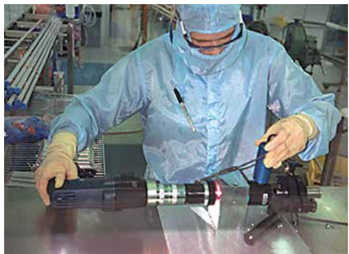
This custom engineered Model 301 has a heavy-duty motor and baseplate, a Quick-lock clamping system and a gear reduction unit to limit the tool bit rotational speed to deal with difficult alloys.
