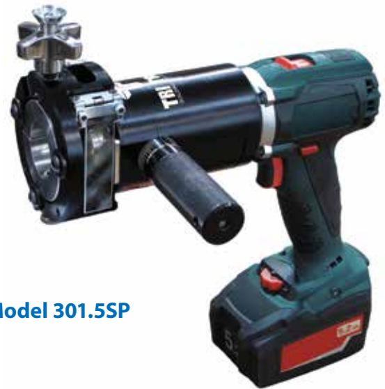
Special saddles for the Model 301SP include dedicated cutouts that correspond with recesses in the tool face to provide the perfect clearances required for squaring gland nut assemblies.
