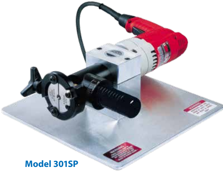
Special saddles for the Model 301SP include dedicated cutouts that correspond with recesses in the tool face to provide the perfect clearances required for squaring gland nut assemblies.
