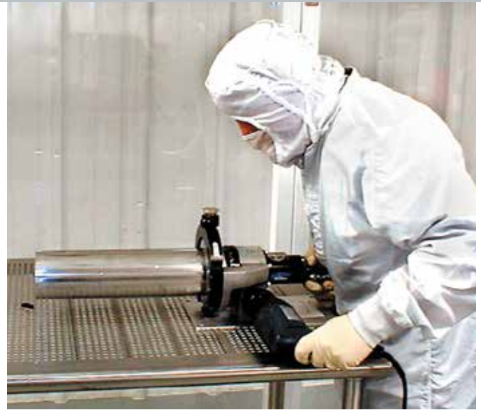
A Model 304 squaring a section of stainless steel tubing in a cleanroom fabrication work area.
