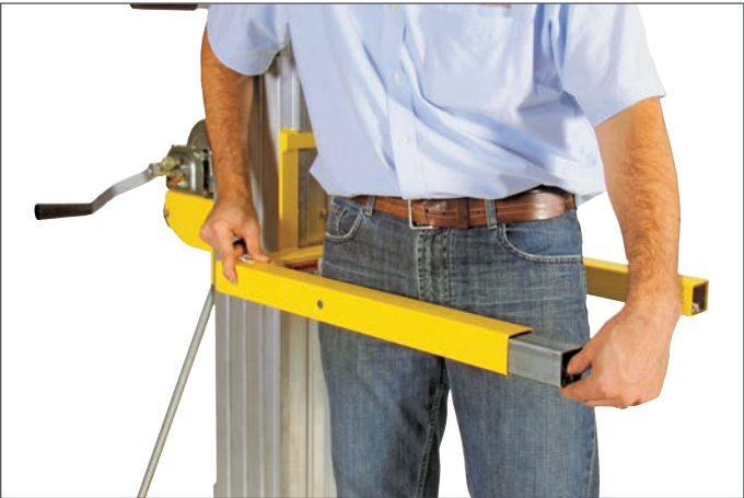
Fork Extensions (Part No. 784695) extend from 23¾" / 59.2 cm - 29⅞" / 75.7 cm at the push of a button. Using extensions reduces capacity to 200 lbs / 90 kg, clearly marked on forks. Another button retracts them for compact storage inside the forks, ensuring quick, convenient adjustment.
