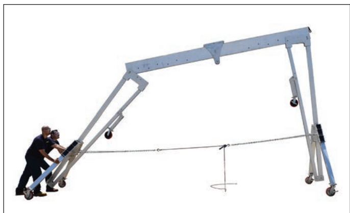
Operate the ratchet on the second A-frame until it can be pushed into place.
