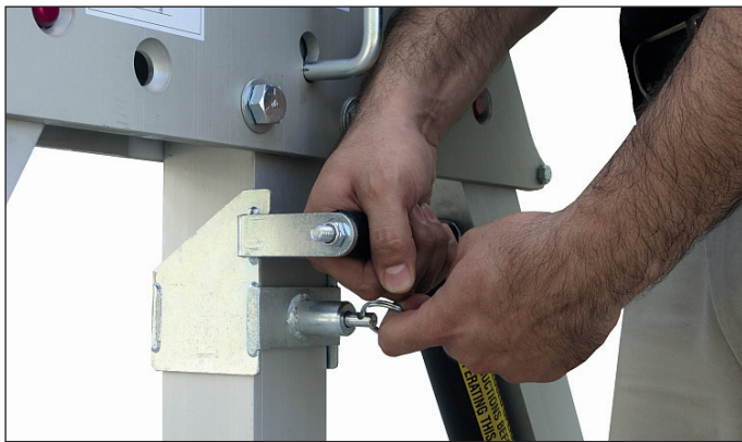
Adjust the mast lift lever with the spring-loaded positioner to a comfortable lifting position.
