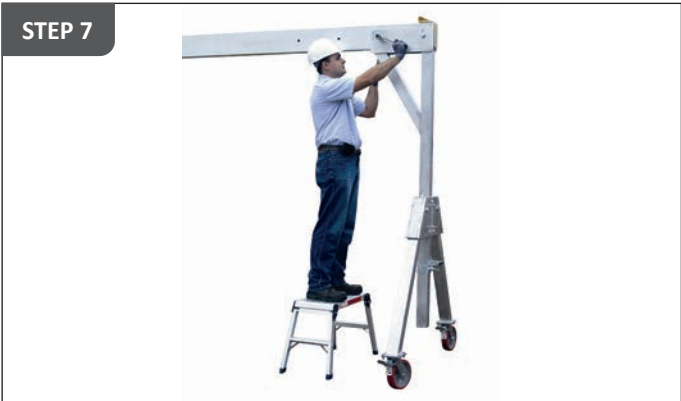
Insert the pins and tighten everything
