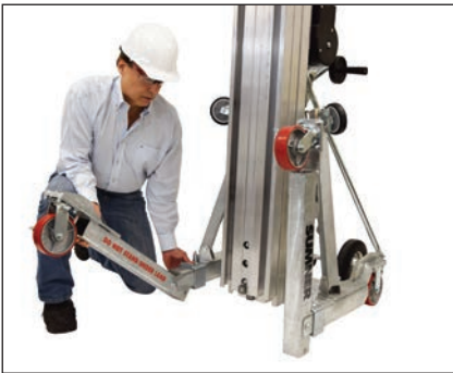
Spring-loaded positioner unlocks legs, allowing them to fold for storage. Roller wheels under each leg enable easy movement in storage position.
