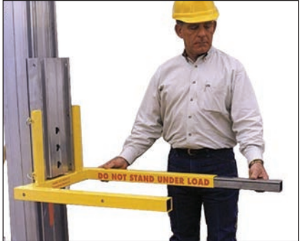
Fork Extensions (Part No. 783691) extend forks from 28 - 42" / 71 - 106 cm at a button press, reducing capacity to 200 lbs / 90 kg. Another button retracts them for internal storage.
