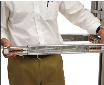
Fork extensions add 8" / 200 mm length with a button press, store inside forks, support 450 lbs / 205 kg. Part 783163.
