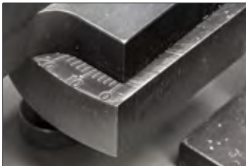
Angle Setting Scale
