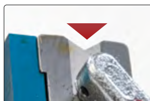
Machined V-Groove For holding round & flat stock.
