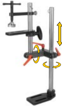
APC250 (18"): Height and angle adjustable with a rotating clamp head; height range 3.9"~26" for advanced and non-square setups
