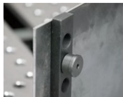
Magnet keeps sheet metal in vertical position
