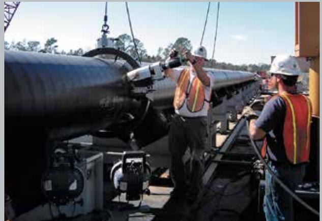
This Clamshell lathe has been configured to perform precision, in-line weld-profiling to strengthen weld joints for offshore platform tendon legs.
