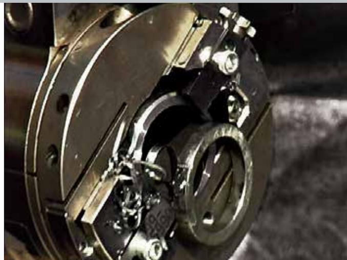
An SBCM clamshell has just completed the severing of a training coupon. This machine had been configured for a sequential sever and bevel operation. You can see the top most bit has completed the sever and the severed end is falling away. The bit at the bottom is in the process of generating the bevel to the specified depth.
