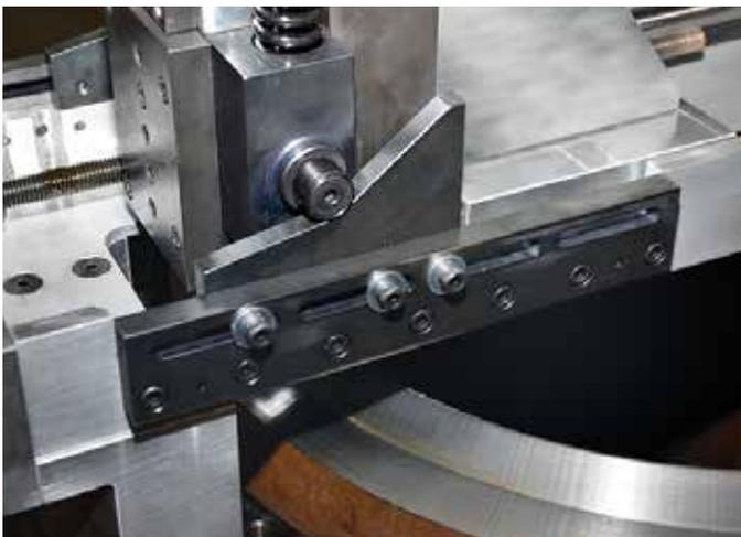
*The simple and reliable spring-loaded TTM tool module follows a pair of adjustable templates, transferring the traced shape precisely to the pipe end.*
