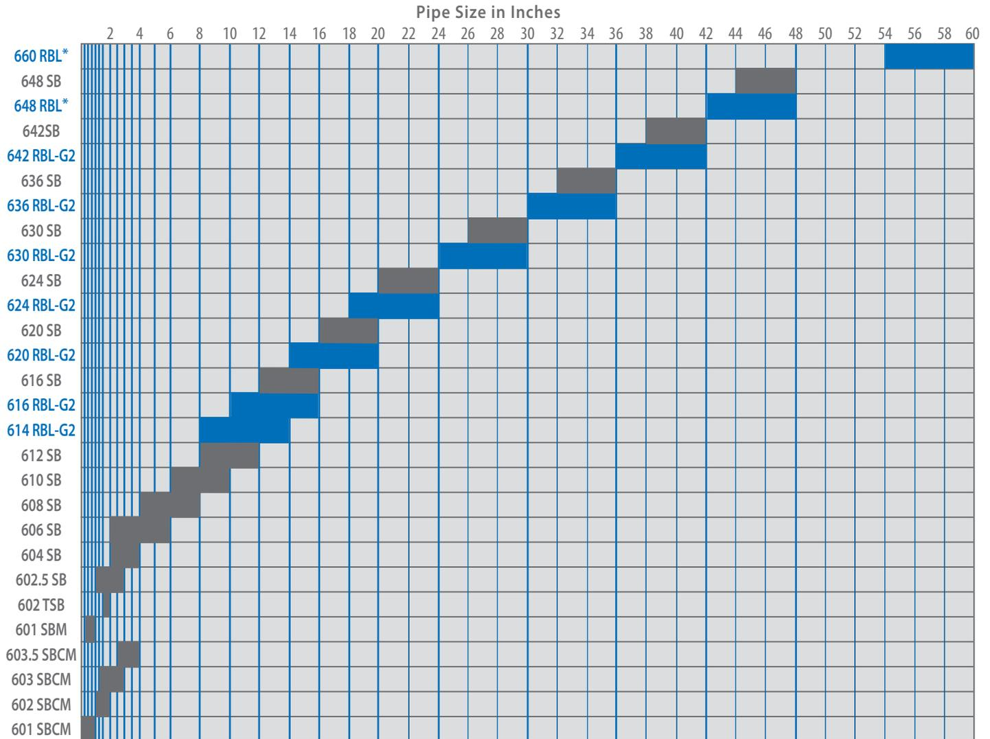
*\* The 648 - 660 RBL clamshell lathes include cutting modules and surface treatments that are different from those included with the 614-642 RBL-G2 type clamshell lathes. When using optional or custom accessories with 600 Series lathes, the actual cutting range may be extended wider, higher, or lower than those shown. Refer to the Specifications on Page 18 of this brochure, or contact your Tri Tool technical sales representative for more information.*
