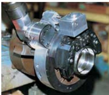
*A small SB lathe fitted with a cut-off wheel module performs "chipless" cutting of thin-wall tubing.*
