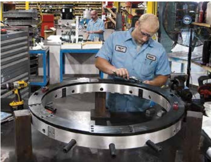
*Each returning Clamshell is thoroughly inspected and adjusted by expert technicians, ensuring "like new" operation and ready-to-rent status.*
