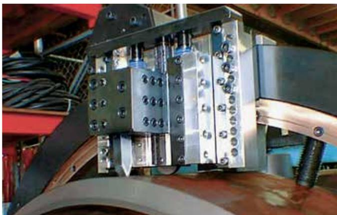
An OD Tracking Module accessory being utilized on a large SB clamshell. The Tracking Module compensates for out-of-round conditions by "reading" the pipe shape with a wheel, automatically adjusting cut depth.
