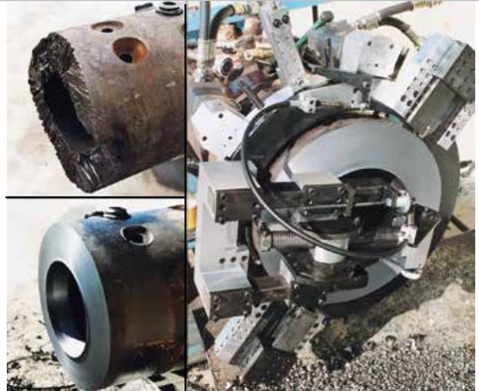
*A 600 RBL series split frame lathe configured with a single point machining module generating a precision heavy wall "JPrep" weld profile and counterbore on a flame-cut pipe end.*
