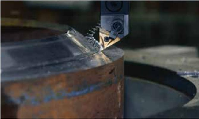
*Designed to utilize readily available and easy to source components, the Template Tracer Module cuts with standard tool holders and inserts.*
