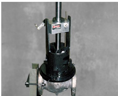
VM8000 Globe and Control Valve Repair
