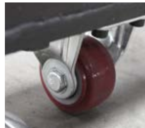
Two casters for quick repositioning of manipulator.
