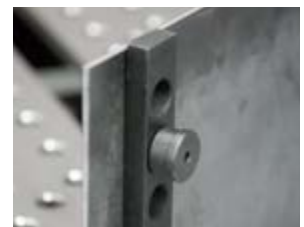
Magnet keeps sheet metal in vertical position
