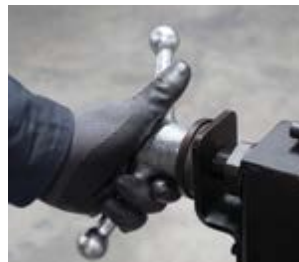
Two large handles for quick & easy adjustment of rotary axis
