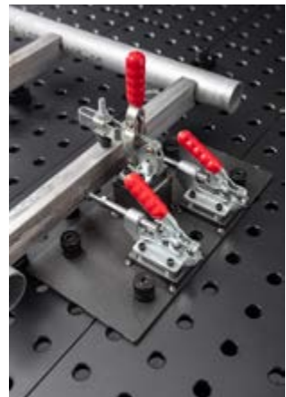
Mounted with Straight Edge Stop attachment and Ball Lock Bolts.
