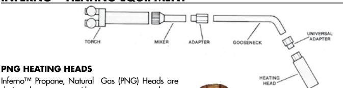
Inferno™ Propane, Natural Gas (PNG) Heads are designed to operate with propane or natural gas. Shells are machined from solid copper bar stock. Internals are machined from brass which is press fit and pinned to prevent separation during backfire. A wide selection of sizes delivers from 200,000 to 1,200,000 BTU's.
