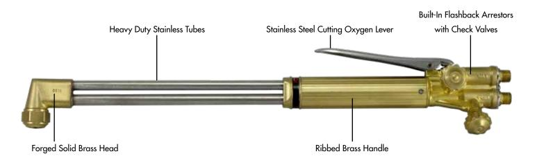
Flame Tech's Scorpion 2621-90 torch is designed for heavy duty hand held applications for the fabshop, foundry or scrap yard environment where up to 8" cutting is required. Universal mixer provides optimal performance with any fuel gas.
