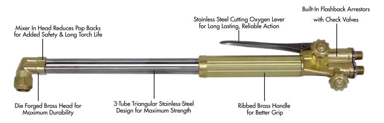
Flame Tech's Scorpion 921-90 torch is designed for heavy duty hand held applications for the fabshop, foundry or scrap yard environment where up to 5" cutting is required. Universal mixer provides optimal performance with any fuel gas.
