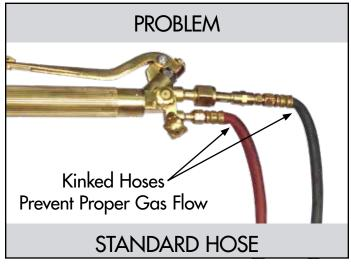
Cutting failures occur when hoses are kinked and gases can not flow properly. Extensive kinking shortens hose life by creating cracks and dangerous gas leaks.
