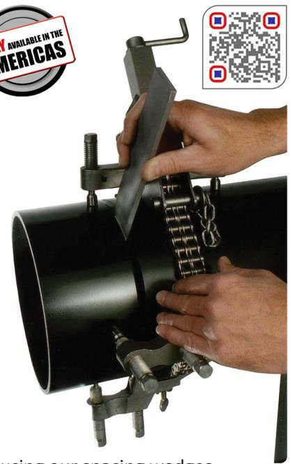
Weld gap can be quickly set using our spacing wedges.
