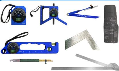
Fit-Up Pro offers several tools specific to pipe layout. A new pocket level and fitters torpedo level are made from aircraft aluminium balancing light weight and durability. A newly designed pipe centering tool adds magnets for hands free use and comes with a right angle square and handy ruler markings, and our line of radius markers is great for laying out a radius or circles up to 100 inches.
