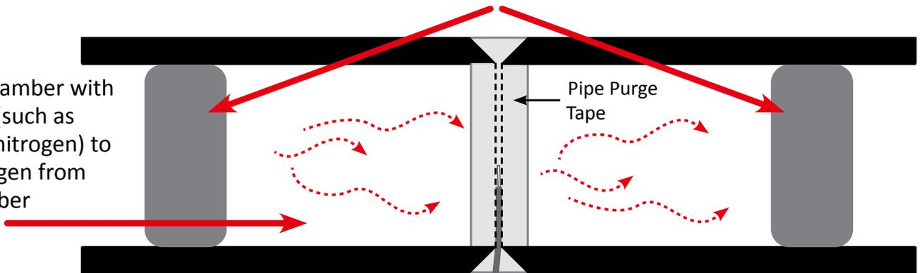
3. Use a weld purge monitor to recognize when the required level of oxygen has been met
