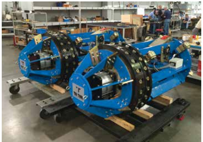
Above, a pair of ILUC 4648 Internal Line-Up Clamps show both the blades and roller system for guidance and reliable positioning within the pipe section.
