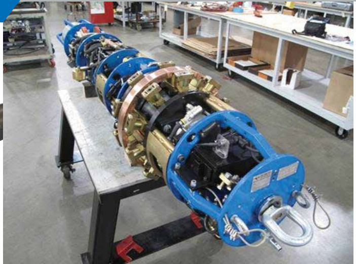
This ILUC 1820 is configured for vertical operation with a strong lifting eye and cable controlled braking system to prevent the clamp dropping down the pipe.
