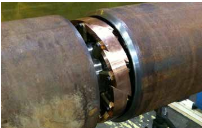
The interlocking copper shoes of this ILUC 1416 are shown in the retracted position that decreases the diameter for unrestricted travel within the pipe ID.
