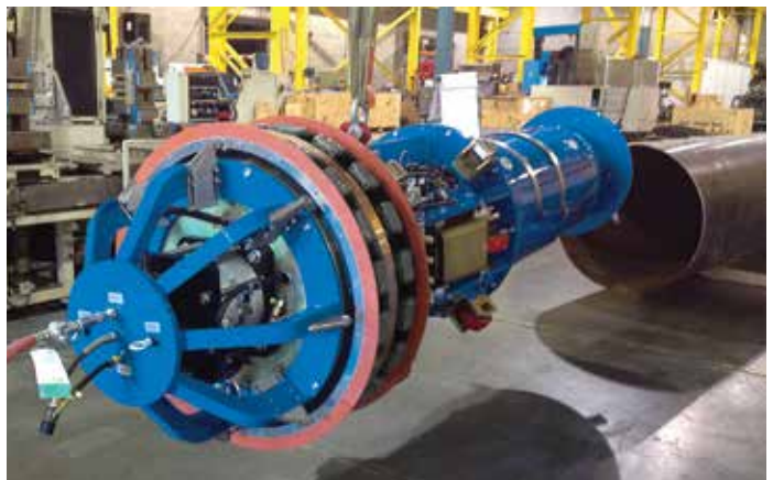
The ILUC 4244 above not only provides precise alignment, it is fitted with purge dams that form a weld gas controlled chamber surrounding the backing shoes.
