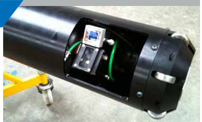
An ILUC mounted VLSM shows both the laser and illuminated video modules.
