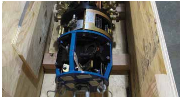
A new CLAMPMASTER Internal Line-Up Clamp ready for deployment.
