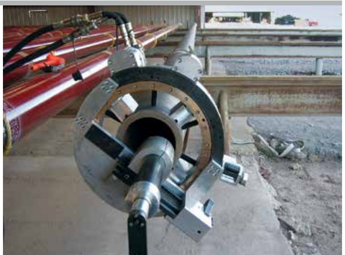
The Tri Tool 600 Series Clamshell provides a stable and secure platform for precision counterboring, an absolute necessity for pipe matching and testing.
