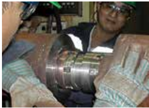
An ILUC 810 used for weld backing on small diameter heavy wall pipe.
