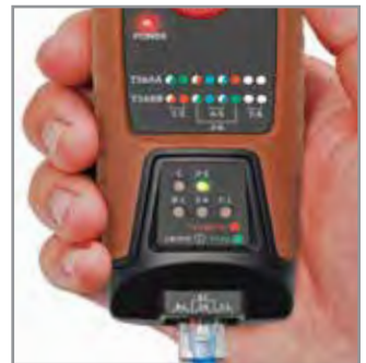
Illuminated LEDs and color wiring reference chart
