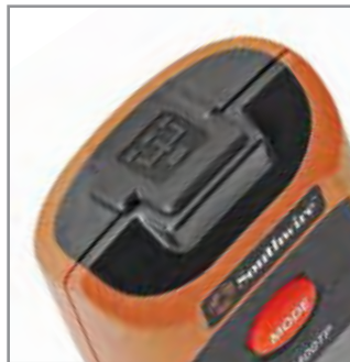
Port covers protect RJ45 ports from dust and debris
