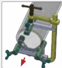
Loosen the main clamp arm.
