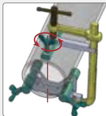
Turn three adjustment screws to preset.
