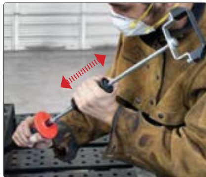
The built-in sliding hammer enables odd direction/position hammering.
