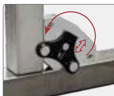
The face plate can be slid out of the boundary edges as edge guide.
