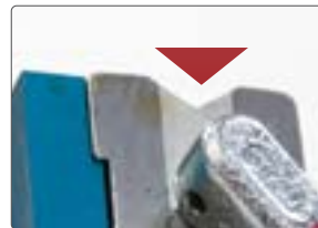
Machined V-Groove For holding round & flat stock.
