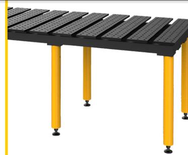
BuildPro Slotted table tops are constructed from 5/8" thick steel plates and feature a 1.7" slot between plates. Top plates are CNC machined with Ø5/8" boreholes that are equally spaced on a 2" grid pattern. All Slotted tables feature patented reversible and self-locating tabletop plates.
