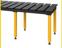
BuildPro Slotted table tops are constructed from 5/8" thick steel plates and feature a 1.7" slot between plates. Top plates are CNC machined with Ø5/8" boreholes that are equally spaced on a 2" grid pattern. All Slotted tables feature patented reversible and self-locating tabletop plates.
