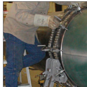
Heavy duty jackbars for arduous aligning and reforming jobs
