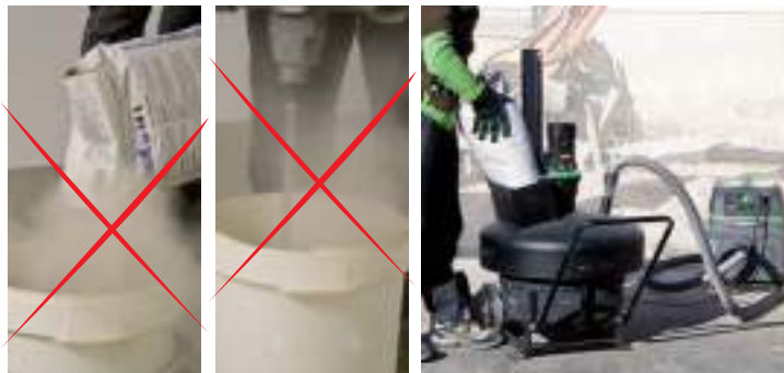
Pouring inlet tube and integrated dust extraction port reduce airborne dust while adding and mixing materials.
