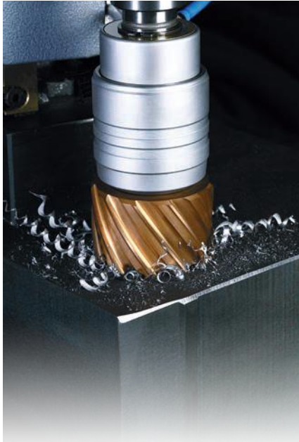
Annular Cutter Recommended Revolutions Per Minute Recommended Feed Rate: .002 - .004 inches per revolution
