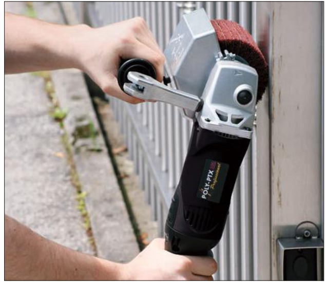
Satin finishing using interleaf fleece wheel.
