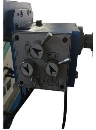
Gear box feeder
