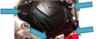
B. If removing the plastic clutch case cover you can remove the OEM brake light switch mounting bracket by removing the (2) 8 mm bolts on the inside of the frame. You will also be required to replace 3 of the case mounting bolts with 28mm bolts (Shorter)
