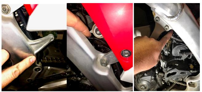
**3.** Disconnect the OE kickstand sensor wiring at the connection. Disconnect by compressing the release at the back of the connector on the chain side of the engine. Use slight tension to pull the connection apart while connection release tab is compressed. Place OE wiring out of the way.
