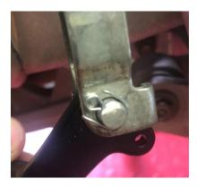
**10.** Install the new brake pedal assembly by installing the 8mm Allen pivot bolt, making sure the steel washer is installed between the frame and the brake pedal. Torque to OEM spec. Reinstall the OEM return spring.
