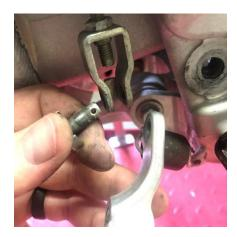
8. Remove brake pedal bushing seal from OEM brake pedal, install seal carefully into the new brake pedal (use light grease)
