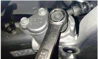
Install the hydraulic banjo brake light switch with a crush washer on both sides of the brake line mounting head. Hold the brake light switch wiring above the body and rotate with the banjo while tightening. \*\*\*NOTE\*\*\* Do not twist the brake light switch wires while tightening the brake light banjo as this can cause damage the wiring or brake light switch. Tighten to OEM torque spec. (14mm)
