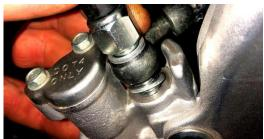
It may be necessary to remove the brake fluid reservoir cap to correctly tighten/torque the brake light switch banjo, this is fine as the next step is to bleed the system.
