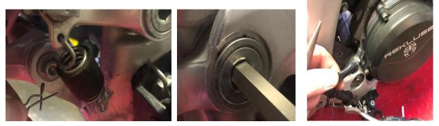
7. Remove the brake pedal return spring, then continue by remove the brake pedal engagement pin, by using pliers to remove the cotter pin/safety pin on the frame side of the brake pedal engagement arm.
