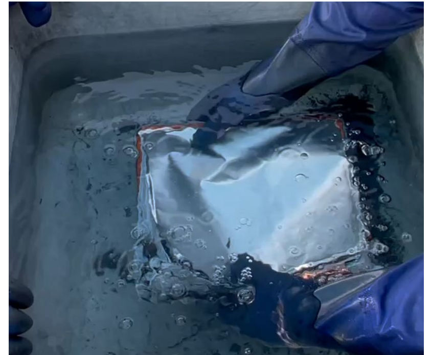
Battery cell taken apart in FSS
