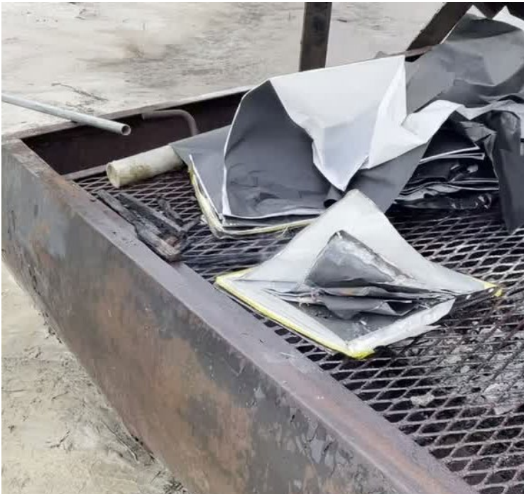
Battery cell opened without FSS
