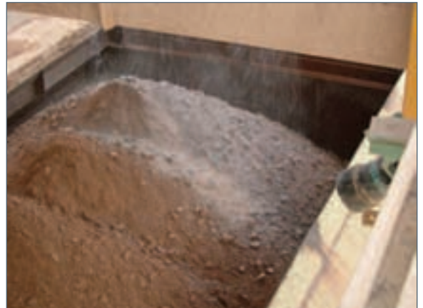
RAIL TRUCK LEVEL FOR WATER SPRAY CONTROL
