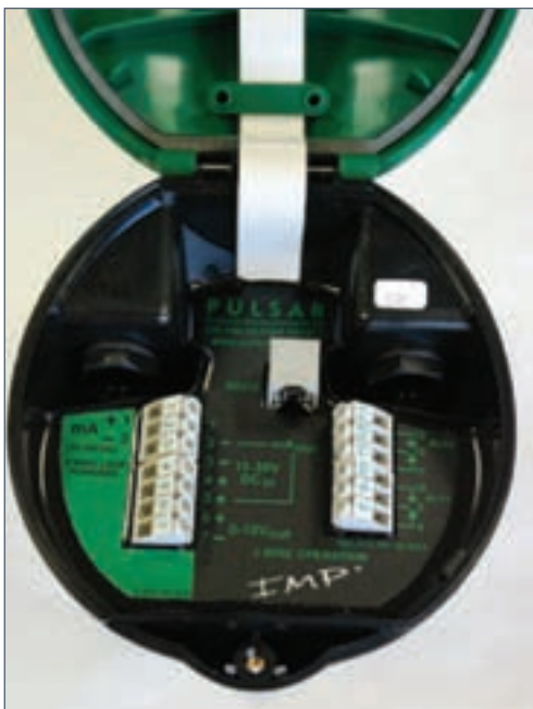
INSIDE OF STANDARD 2/3 WIRE IMP
