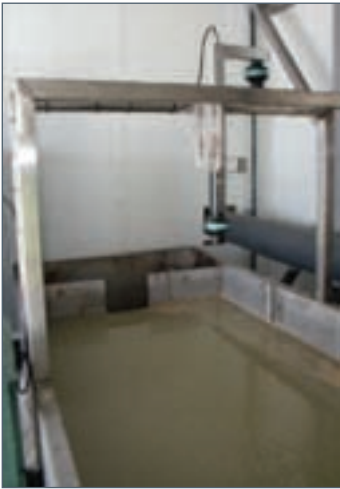
RECTANGULAR WEIR and DUET TRANSDUCER
