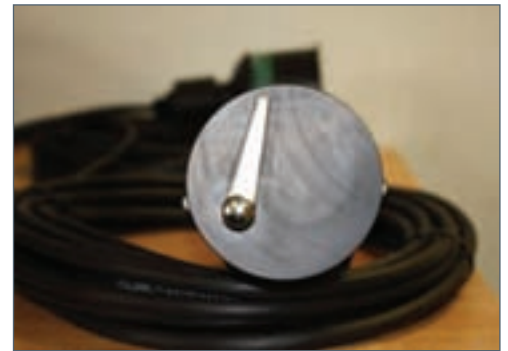
FRONT VIEW OF VIPER FACE SHOWING WIPER
