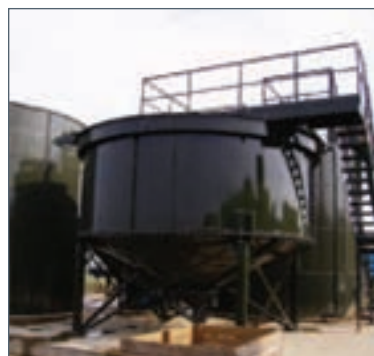
BLACKBOX ON MIXING TANKS WITH AGITATORS
