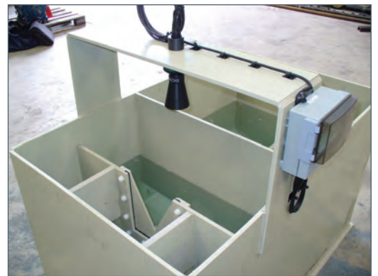
FLOW BOX WITH A V-NOTCH WEIR and dBMACH3
