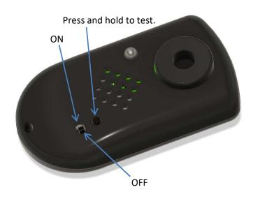
The CM-2010 can be left ON continuously and the battery will last many years. Check the battery before use by: turning ON, and **holding** the test button (up to 4 seconds may be necessary). The alarm will not flash and sound if the battery needs replacing.
