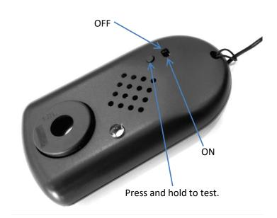
We recommend the CM-2010 be left ON continuously; the battery will last many years. If the battery needs replacing the alarm will give a quick chirp and flash every minute. You can also check the battery by **holding** the test button (up to 4 seconds may be necessary). The alarm will not flash and sound if the battery needs replacing.
