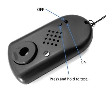
We recommend the CM-2010 be left ON continuously. Under normal operating conditions the battery will last up to 5 years. When the battery needs replacing the alarm will give a quick chirp and flash every minute. You can also check the battery by holding the test button (up to 4 seconds may be necessary). The alarm will not flash and sound if the battery needs replacing.
