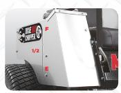
Fuel Sight – Check how much fuel is left in the tank without removing the cap.
