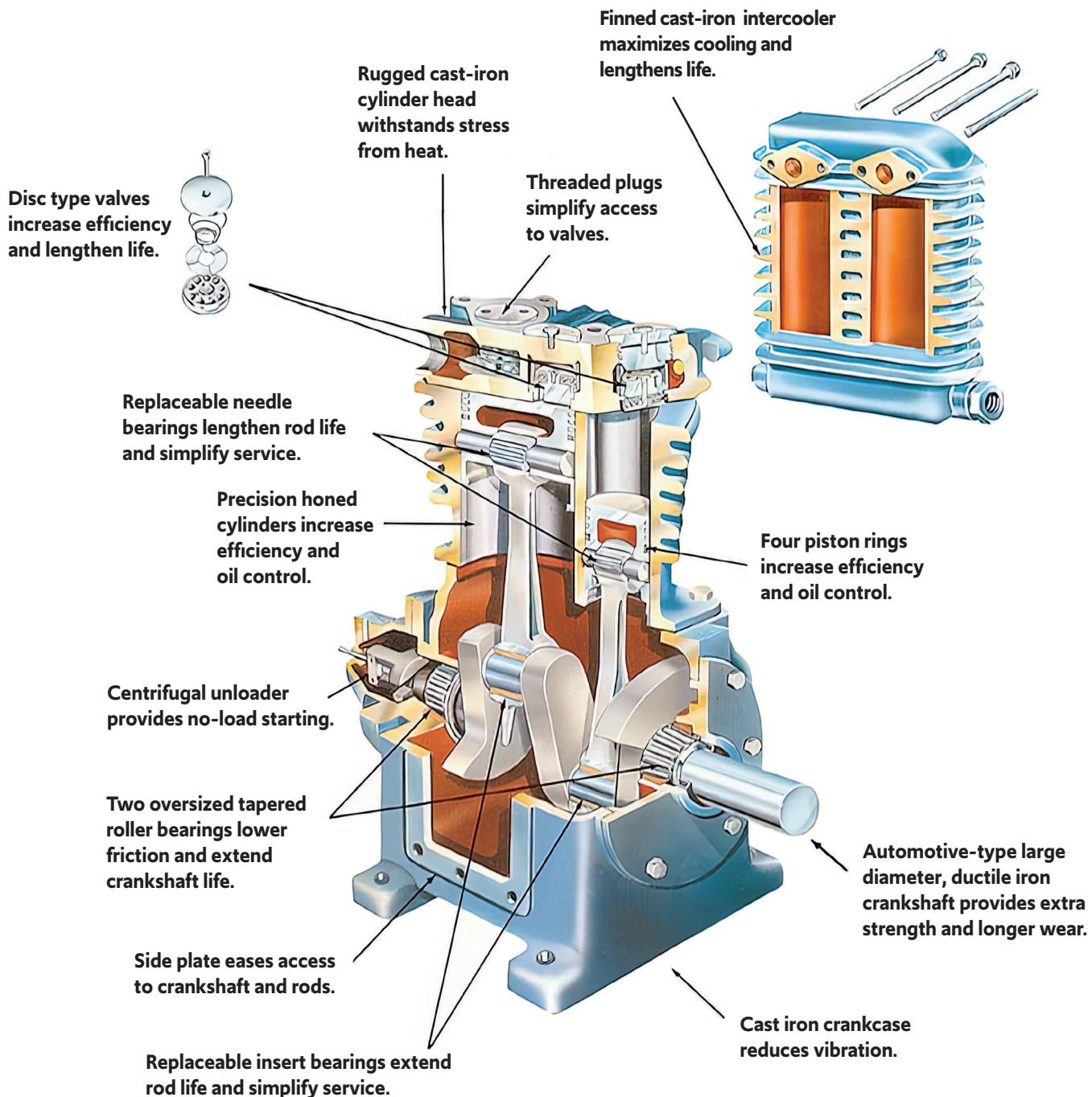
Saylor-Beall uses piston rings specifically designed for two-stage air compressors. They have a special taper and an overlapping joint to eliminate ring gap. This ensures less compressed air blow-by and reduces oil carry-over.
