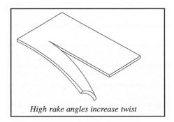
Although twist can be caused by internal stresses in the material and dull knife blades, it is primarily created via the rake angle of the upper knife blade and the width of the drop piece. High rake angles will substantially increase the twisting action of the material during the shearing process.
