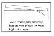
the shearing process. Once again, it is most prevalent when shearing long, narrow strips. It is caused by deficiencies or stresses in the material and shearing at higher rake angles.
