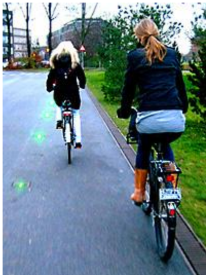
Figure 19: Example of LED Embedded Lighting 30
