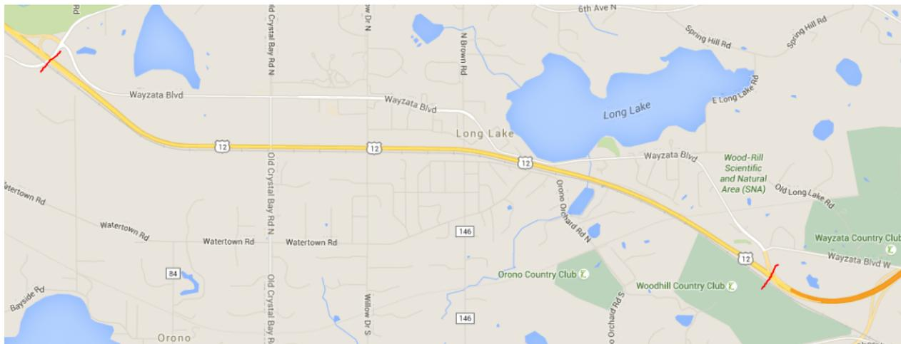
Segment N is 4.02-miles in length and is bounded to the west by CSAH 6 (see Figure 5-50 for a visual of the segment). The segment has two-lanes and is mostly classified as being rural, but also has some sections with curb and gutter.
