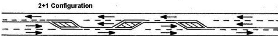
**Figure 5-16: 2+1 Passing Lane Section<sup>34</sup>**
