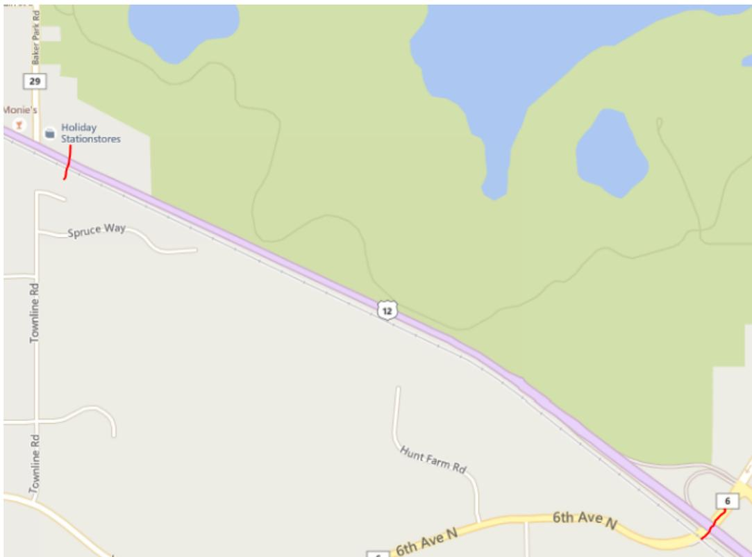
Segment M is 1.54-miles in length and is located between the City of Maple Plain and CSAH 6 (see Figure 5-46 for a visual of the segment). The segment is classified as a two-lane, rural highway. The FAR for Segment M was 3.66 crashes per 100 MVM, which exceed both the state average (1.57 crashes per 100 MVM) and the critical FAR (1.80 crashes per 100 MVM).
