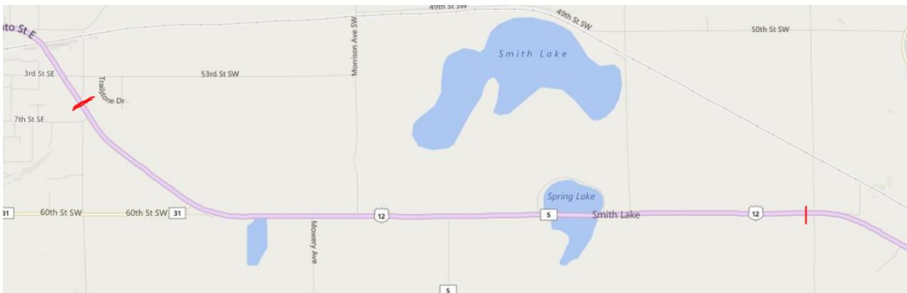
Segment C is located between the Cities of Cokato and Howard Lake. Refer to Figure 5-29 for a map view of the segment. The segment is 4.16 miles long and is primarily characterized as a two-lane rural highway. There is a 0.8 mile portion of the segment that has four-lanes. General corridor-wide and rural segment recommendations should be applied to this corridor. The following paragraphs further explain the recommendations listed in Table 1-2 for Segment C.
