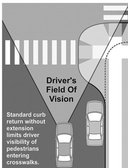
Because installation can be done on a short schedule, curb extensions should be added in the short-term. It is much more effective to install permanent curb extensions, however, if it is not possible to install right away, temporary curb extensions can be created using bollards and pavement markings, as shown in Figure 5-8. Although better than nothing, bollards can become a maintenance burden because they get hit easily and do not create as much physical protection for pedestrians.
