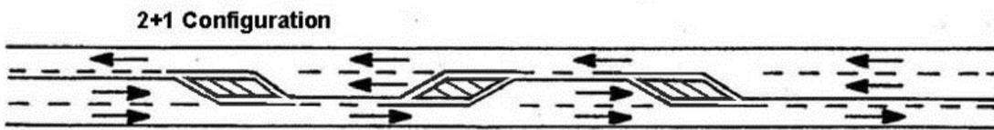
**Figure 5-16: 2+1 Passing Lane Section<sup>34</sup>**
